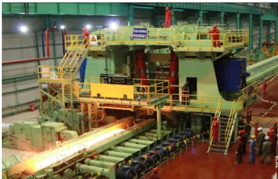
This project was for a greenfield mill that was to be built in China. The mill was designed with the capacity for 1.45 meter wide strip and 3.5 megatonnes/year having 7 finishing stands, a coil box, and 2 roughing mills. The mechanical contractor was Danieli and ABB was the electrical supplier for which IPSS acted as the “technology provider”.
